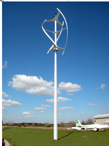
Figure 2.17: QuietRevolution VAWT wind turbine
