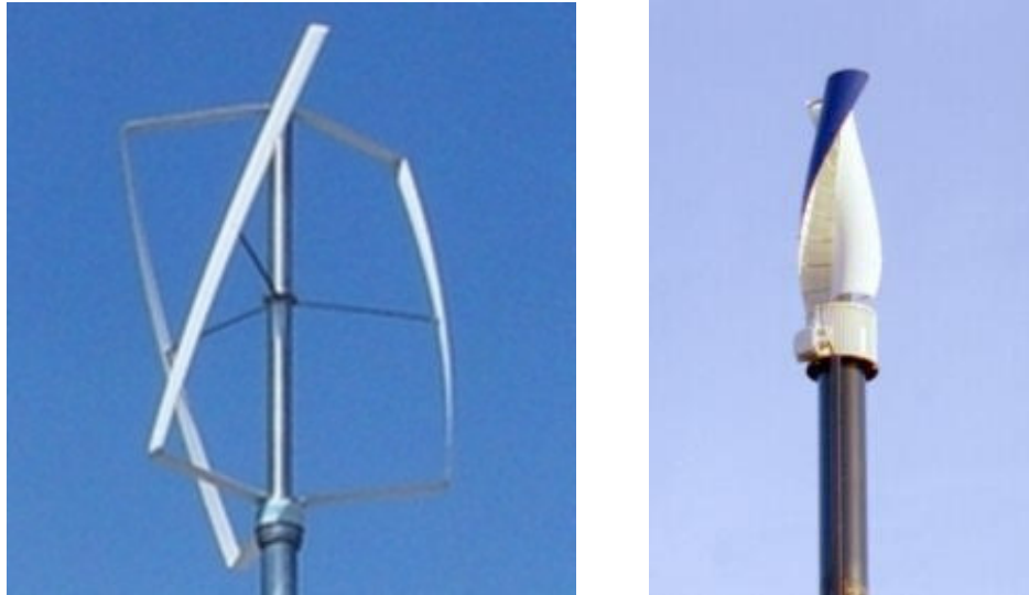
Figure 2.2: Two types of vertical axis wind turbines, a Darrieus (left) and Savonius (right)
