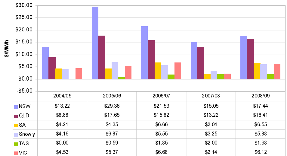
Figure 9 Regional pool price changes between the BAU and a case where the contract cover is lower for all three portfolios
